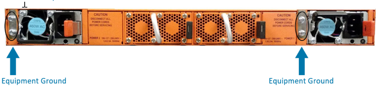
Figure 6 Ground Screws (GigaVUE TA Series-TA10 Shown)
